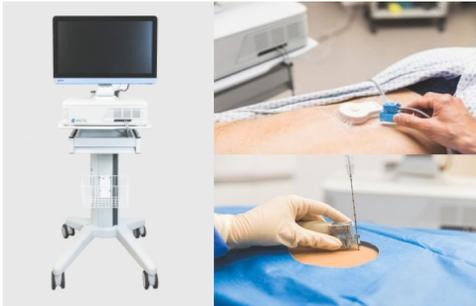
Fig1: IMACTIS hardware. Left image: Touch screen demonstrating images in two planes. Top right: skin fiducial electromagnetic localiser. Bottom right: needle holder with sensor.
